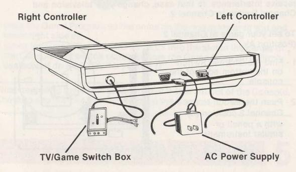
Attach the controllers by plugging them into the terminals on the back of the console. The controller jacks are designed to fit only one way, so do not try to force them into the terminals.
