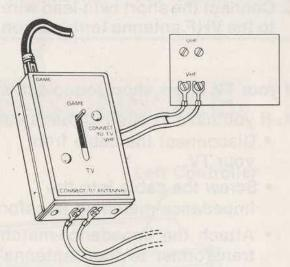
In each of these two cases, you may need to buy an "impedance matching transformer" (also called a "balun coil"). The transformer is necessary only if you do NOT have a flat twin-lead antenna wire. It is available at a nominal cost from your local TV and hifi stores.
